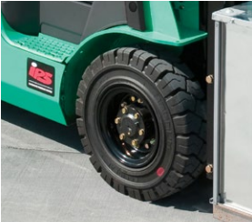
Solid pneumatic dual drive tyres
