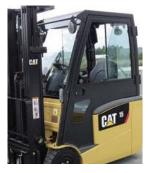
Optional panel cabins available for many trucks in the range, allowing for comfortable external use.
