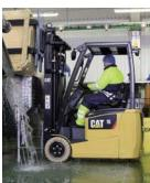
**IPx4 Weather Protection** Ingress Protection against water, in the 48 volt range, allows for dependable operation outside or in contaminated environments.
