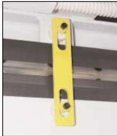
**Mechanical platen lock** to prevent movement.
