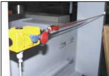
**Perimeter e-stop** safety cable and switch
