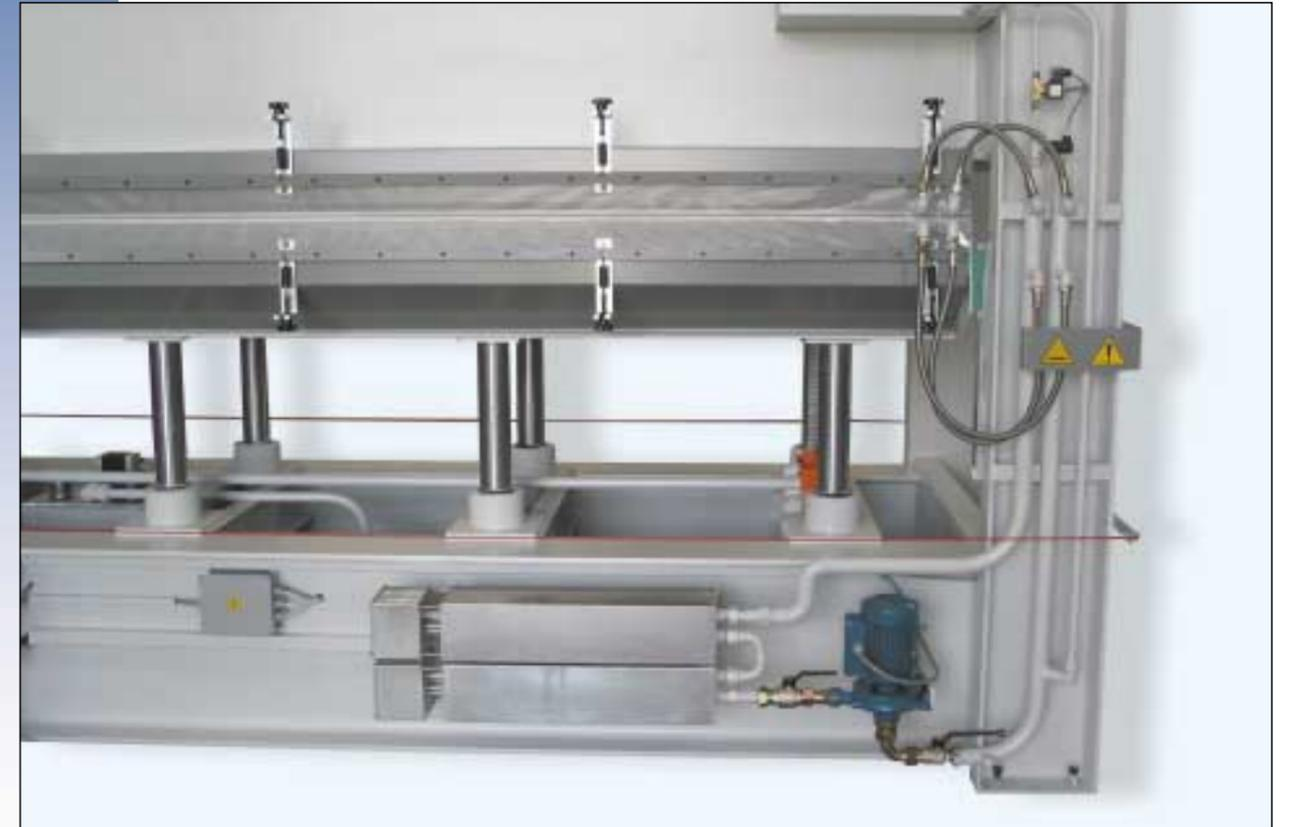
XL press platens can be heated with a variety of heating systems. In some factories central sources like steam, hot water and super heated water may be used to heat the XL's solid steel or fabricated platens. Wood or coal-fired boilers may also be considerations. Since regulating the temperatures of the platens using these fuel sources can be a challenge, in the US we provide either time-tested electric boiler systems or electric platens specifically designed for your press.
