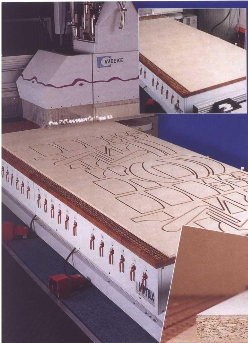
*Non-rectangular shaped parts in a nested sheet of material*
