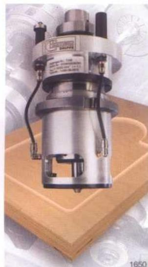
**Routing vertical with tracing ring**
