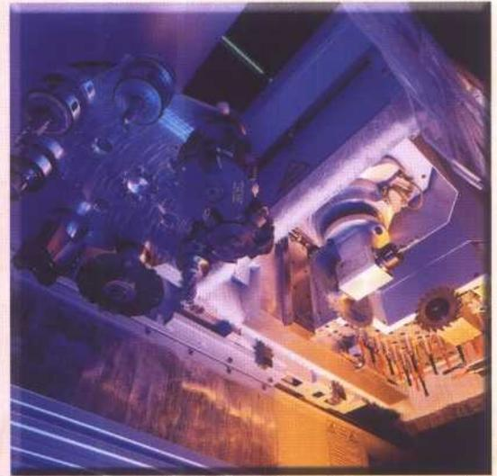
Typical machining head configuration
