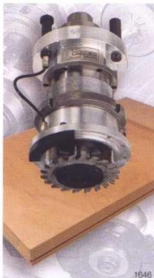
**Routing vertical with tracer shoe**
